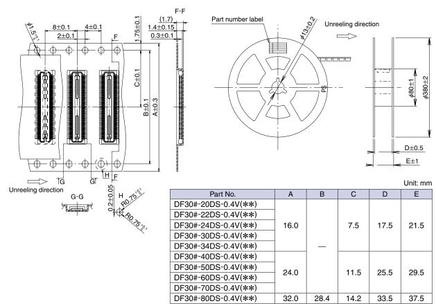
Embossed tape 32mm or wider will have perforated feed holes on two sides.
