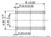
Recommended solder paste thickness: 120  $\mu$ m
