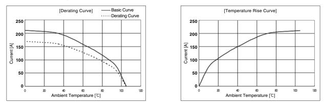
Note 1 : The derating curve is derived from the basic curve multiplied by the derating factor of 0.8.
