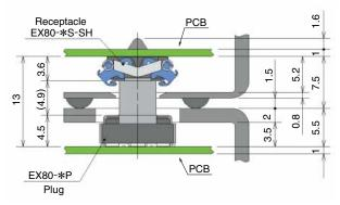
Note: The stacking length between boards of this connector is 13 mm.
