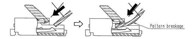
◆ Checking the Locking Condition In the locked condition, make sure that the lock lever is horizontal on the board surface. Do not apply excessive force to it near the 0° position of the lever. Otherwise, the terminals may be deformed. (Allowable force: 1 N or less)
