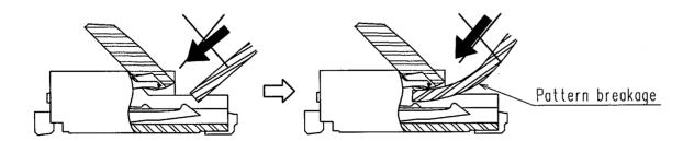
◆ Checking the Locking Condition In the locked condition, make sure that the lock lever is horizontal on the board surface. Do not apply excessive force to it near the 0° position of the lever. Otherwise, the terminals may be deformed. (Allowable force: 1 N or less)
