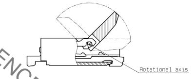
3. The actuator will not open more than 135°. Do not apply any force backward beyond this point. Otherwise, the actuator may come off or break.
