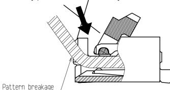
◆Checking the Locking Condition
