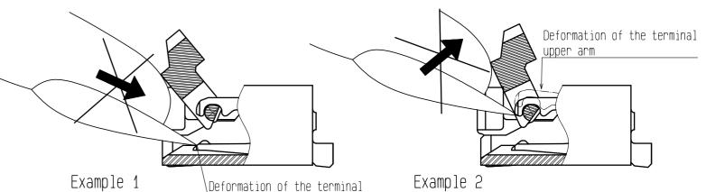
2. The actuator rotates around the rotational axis as shown below. Rotate the actuator.
