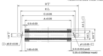
Note 1 The cross-hatched area inside the SMT land may come into contact with the connector contacts and thus care should be taken that the pattern does not extend beyond the SMT land width.
