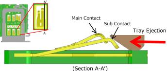
Dual-contact design allows the longer contact to reach tray first, and then the shorter contact smoothly moves along with it.
