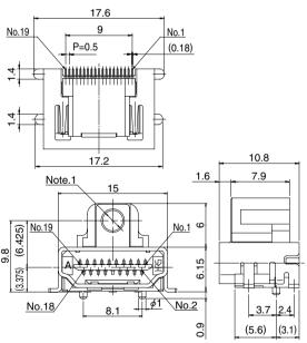
Note 1: Use M3x12mm long pan head self-taping screw.
