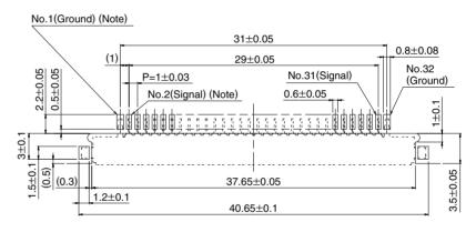
Note: For MDF76LBRW, No.32 (Ground and No.31 (Signal) are on left side.
