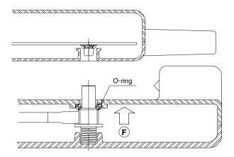
Note 1: When mounting the MS-162-C(LP)-1 make sure that the recommended self alignment distances and angle can be maintained.
