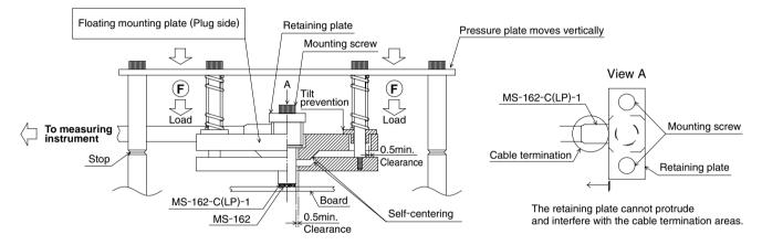
Note 1: When mounting the MS-162-C(LP)-1 make sure that the recommended self alignment distances and angle can be maintained.
