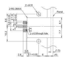
\* Set dimension A to give 50Ω characteristics. Reference example: Glass epoxy t = 1.0 ( $\mathcal{E}$  = 4.8) A = 1.65
