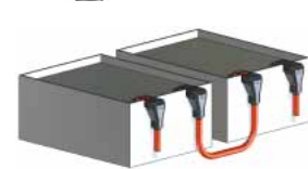
Battery : Flat placement
