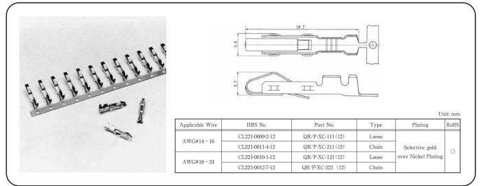
Note\* Loose-piece terminals are available in packs. Each pack contains 100 terminals. Strip terminals are available in reels. Each reel contains QR/P-XC-221 Pin 3,500. QR/P-XC-221 Pin 5,000 terminals.
