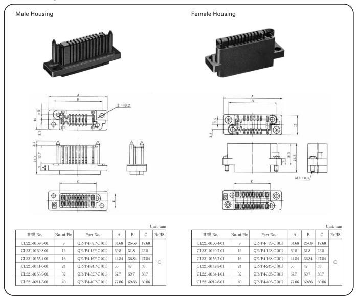
Note: Determine the combinations with the panel so that the mating clearance between the P side and S side is 1.5mm or less.
