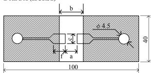
Material: Glass epoxy resin Board thickness: 1.6mm Copper foil thickness: 35μm
