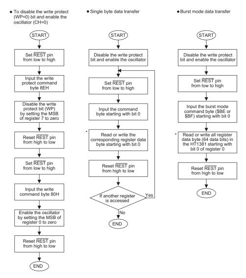
Note: \* In reading data byte from HT1380A/HT1381A register, the first data bit to be transmitted at the first falling edge after the last bit of the command byte is written.
