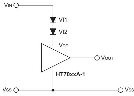
$$\text{Detectable voltage} = V_{f1} + V_{f2} + V_{DET}$$
