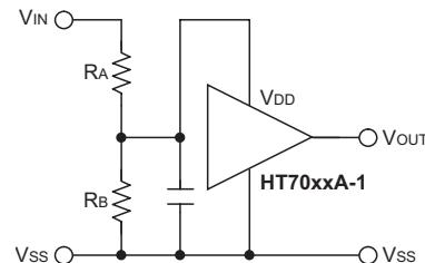
$$\text{Detectable voltage} = (R_A + R_B) / R_B \times V_{DET}$$
