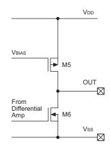
Because of the consideration for minimized power consumption, the max. output current is limited to about 400  $\mu A$  for both source and sink drive. This is believed to be enough for most low power systems, however it is recommended to use the load resistor of >10 k\Omega for normal applications. In case of heavy load driving, an external buffer stage using bipolar transistors is recommended.
