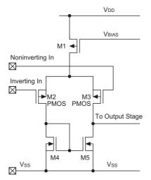
Since the input impedance of PMOS is inherently very high, it can directly couple to high impedance elements without loading effect. For example, coupling to ceramic transducers, integrating capacitor and resistor networks.
