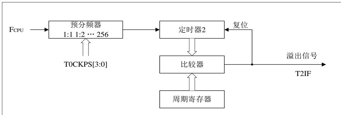
$$\text{Timer2 溢出时间} = (\text{PR2} + 1) * \text{预分频比} / \text{Fcpu}$$
