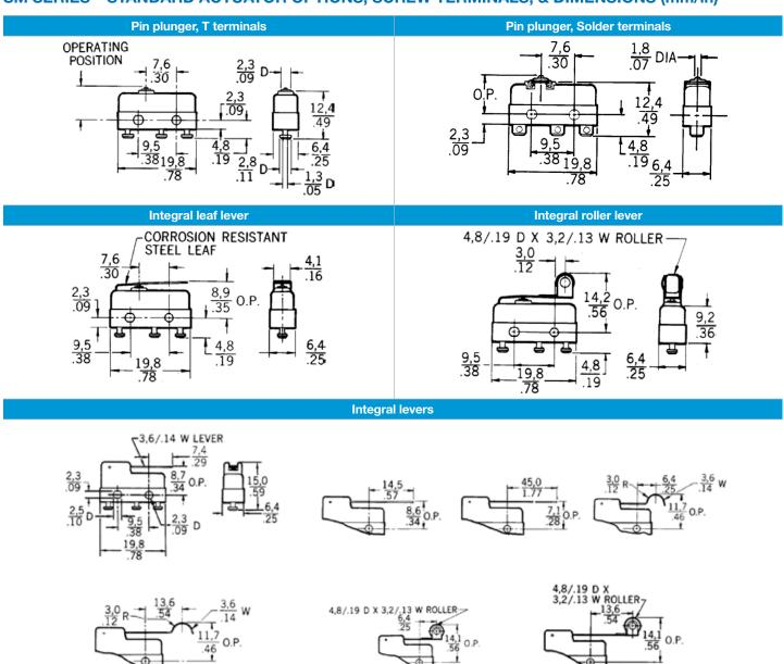
NOTE: The two mounting holes accept pins or screws of 2,21 mm (0.087 in) maximum diameter
