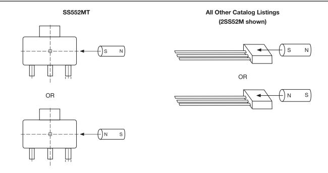
• Operated by magnetic fields (North or South pole) that are parallel to the sensor IC; arrows indicate direction of magnetic flux.
