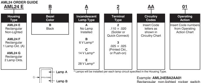
1) The "MICRO SWITCH" identification is shown on this side of the switch housings.
