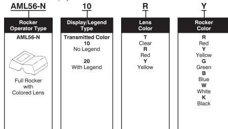
AML56-N rockers have a colored lenticular lens window which extends over the neon lamp.
