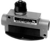
Enclosed Switches Series BZG/BZH: Top Roller Plunger Actuator; 1NC 1NO SPDT Snap Action; 1/2 in - 14NPT conduit
