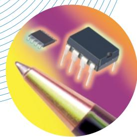
The CLAROCHIP CC9317 digital trimmer is a 7-bit nonvolatile DAC designed to replace mechanical trimmers. It includes a unity-gain amplifier to buffer the DAC output and enables V<sub>OUT</sub> to swing from rail to rail.
