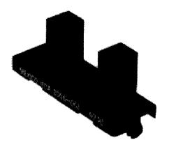
The HOA2006 consists of an infrared emitting diode facing an Optoschmitt detector encased in a black thermoplastic housing. The photodetector consists of a photodiode, amplifier, voltage regulator, schmitt trigger, and an NPN output transistor with a 10 K ohm (nominal) pull-up resistor. The buffer logic provides a high output when the optical path is clear, and a low output when the path is blocked. Both emitter and detector have 1,52 mm (0.060 in.) x 1,52 mm (0.060 in.) vertical apertures.
