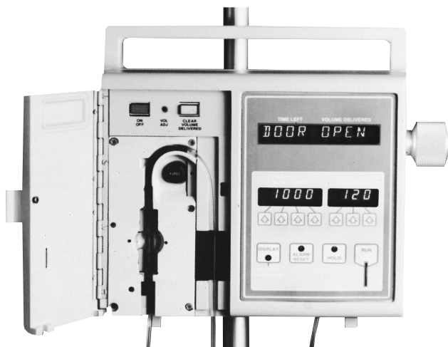
MML medical application. Intranvaneous fluid flow controller automatically dispenses fluids for medications, therapy, and nutrition.
