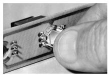
A ¼-turn applied clockwise to the receptacle locks it in the printed wiring board and establishes the electrical connection.
