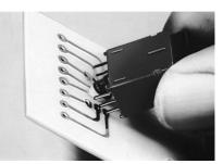
Seat housing on printed wiring board, with LED projecting into hole at the base of the housing.
