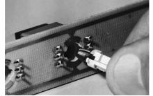
1. Insert the LED/PWB receptacle assembly through a hole in the printed wiring board.
