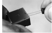
1. Assemble LED to MML44 indicator, with the LED terminals protruding through assembly slot in the middle of housing base.
