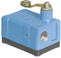
Enclosed Switch Series OP: Side Rotary, Fixed lever length with steel roller, High Temperature, 1NO 1NC Snap Action SPDT, CW actuation
