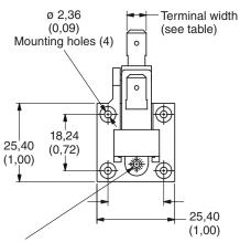
Adjustable Models Only Adjustment screw 1,98mm (,078) Hex socket – clockwise to increase actuation point, counterclockwise to decrease actuation point
