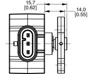
Figure 4. RTP Series Mounting Dimensions (For reference only: mm [in].)
