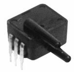
The SDX series sensors provide a very cost effective solution for pressure applications that require small size plus performance. These calibrated and temperature compensated sensors give an accurate and stable output over a 0 °C to 50 °C [32 °F to 122 °F] range. This series is intended for use with non-corrosive, non-ionic working fluids, such as, air and other dry gases.
