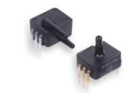
The SDX series sensors provide a very cost effective solution for pressure applications that require small size plus performance. These calibrated and temperature compensated sensors give an accurate and stable output over a 0°C to 50°C temperature range. This series is intended for use with non-corrosive, non-ionic working fluids such as air, dry gases and the like.
