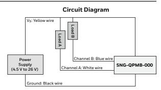
Note: The load resistor values should be such that the output current does not exceed the maximum load current of 40 mA.
