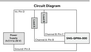
Note: The load resistor values should be such that the output current does not exceed the maximum load current of 40 mA.
