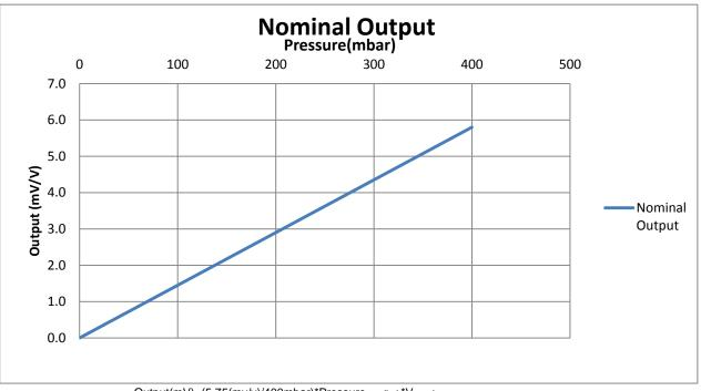
Output(mV)=(5.75(mv/v)/400mbar)\*Pressure applied \*Vsupply
