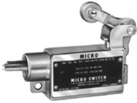
Prewired Enclosed Switches Series BZLN: Top Roller Arm Actuator; SPNO; No. 14 wire leads with 1/2 in - 14NPSM conduit hub; Right-hand Actuator
