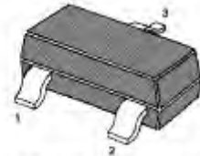
Marking Code: A7 SOT-23 Plastic Package
