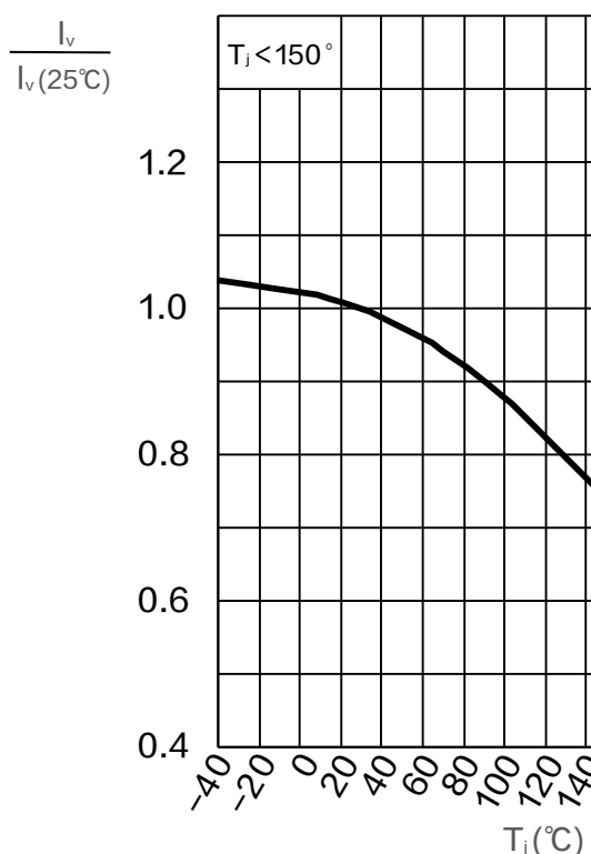
相对发光强度 / Relative Luminous Intensity I_v / I_v(25^\circ C) = f(T_j); I_f = 1000 mA
