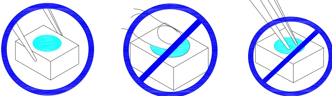
2.The outer diameter of the SMD pickup nozzle should not exceed the size of the LED to prevent air leaks. The inner diameter of the nozzle should be as large as possible. A pliable material is suggested for the nozzle tip to avoid scratching or damaging the LED surface during pickup. The dimensions of the component must be accurately programmed in the pick-and-place machine to insure precise pickup and avoid damage during production.
