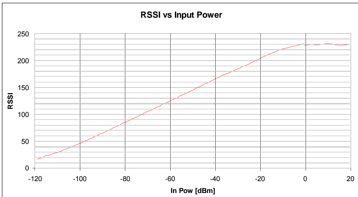
Figure 31. RSSI Value vs. Input Power
