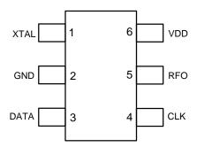
Figure 2. CMT2110/17A Pin Assignments
