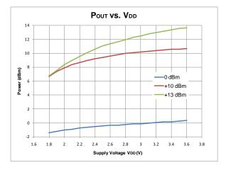
Figure 7. Output Power vs. Supply Voltages, F<sub>RF</sub> = 433.92 MHz
