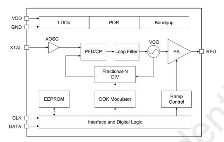
Figure 11. CMT2110/17A Functional Block Diagram
