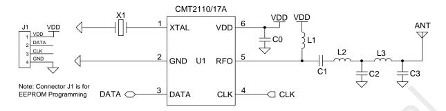
Figure 10. FCC/ETSI Compliant Application Schematic
