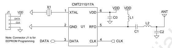
Figure 9. Low-Cost Application Schematic
