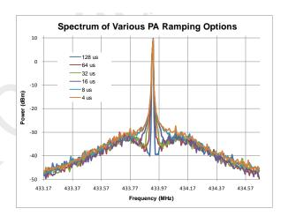
Figure 6. Spectrum of PA Ramping, SR = 9.6 ksps,  $P_{OUT}$  = +10 dBm
