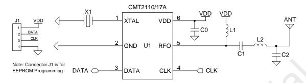
Figure 1. CMT2110/17A Typical Application Schematic
