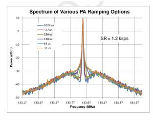
Figure 8. Spectrum of PA Ramping,  $SR = 1.2 \text{ ksps}, P_{OUT} = +10 \text{ dBm}$
