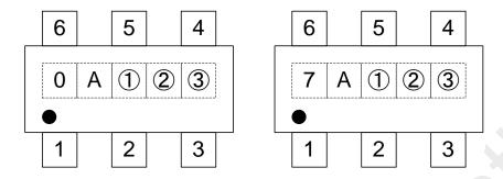
Figure 25. CMT2110A (Left) and CMT2117A (Right) Top Marking
