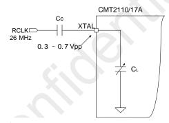
Figure 14. XTAL Circuitry and Crystal Model
