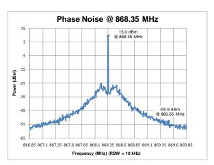
Figure 4. Phase Noise,  $F_{RF} = 868.35 \text{ MHz}$ ,  $P_{OUT} = +13 \text{ dBm}$ , Unmodulated
