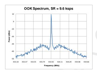
Figure 5. OOK Spectrum, SR = 9.6 ksps,  $P_{OUT} = +10 \text{ dBm}, t_{RAMP} = 32 \text{ us}$
