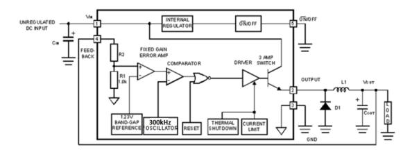
Figure 1. Block Diagram and Typical Application
