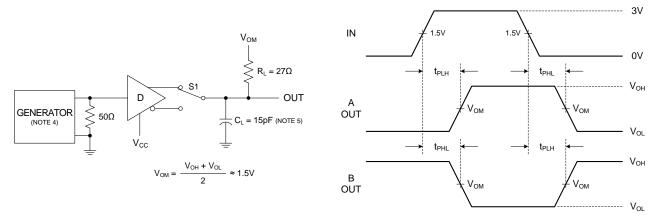
Fig. 4. Driver Propagation Delay
