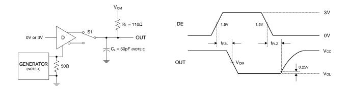
Fig. 6. Driver Enable and Disable Times, Output Low
