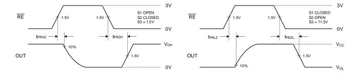
Fig. 8. Receiver Enable and Disable Times
