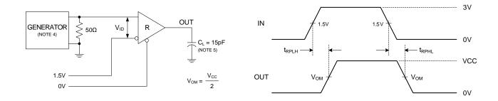
Fig. 7. Receiver Propagation Delay
