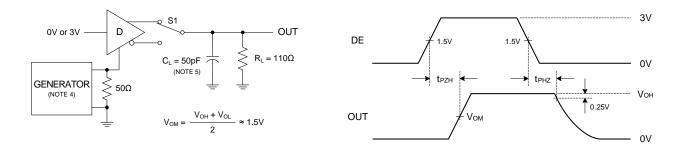
Fig. 5. Driver Enable and Disable Times, Output High
