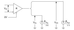
Fig. 1. Driver  $V_{\text{OD}}$  and  $V_{\text{OC}}$
