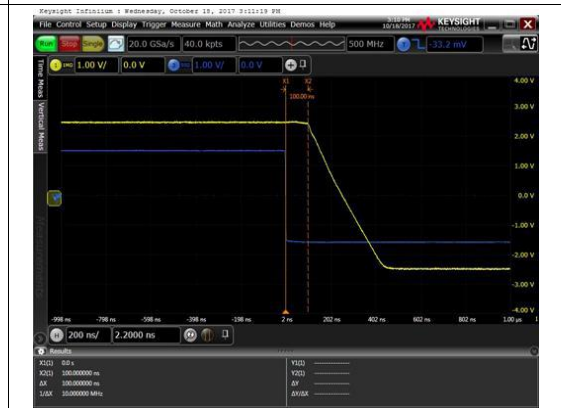
Voltage: 1V/div, Time: 200ns/div V_s = 5V, V_{IN} = 2V, R_L = \text{Open}, G = 3 Figure 24. Negative Overload Recovery
