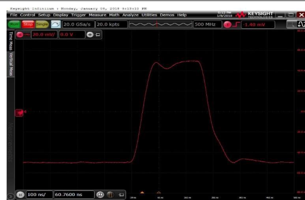
Voltage: 20mV/div, Time: 100ns/div V_s = \pm 15V , R_L = 2K , C_L = 100pF , G = 1 Figure 25. 100mV Signal Step Response
