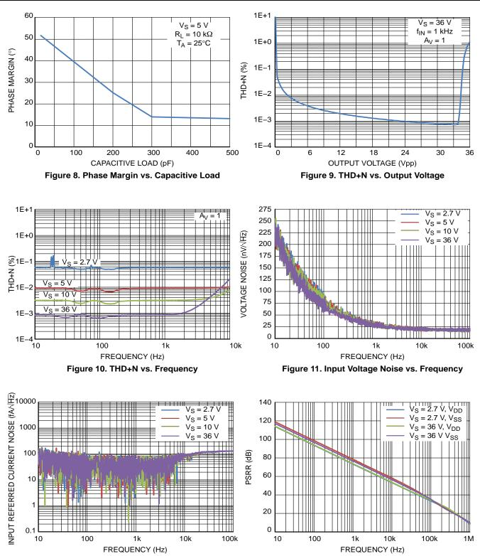
Figure 12. Input Current Noise vs. Frequency
