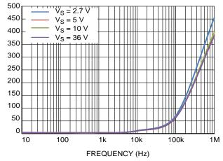
Figure 25. Open Loop Output Impedance
