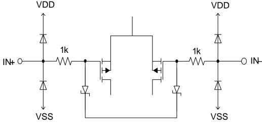
Figure 29. Differential Input Pair
