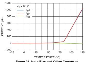
Figure 21. Input Bias and Offset Current vs. Temperature
