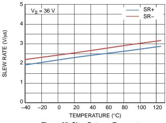
Figure 28. Slew Rate vs. Temperature
