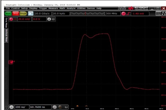
Figure 25. 100mV Signal Step Response
