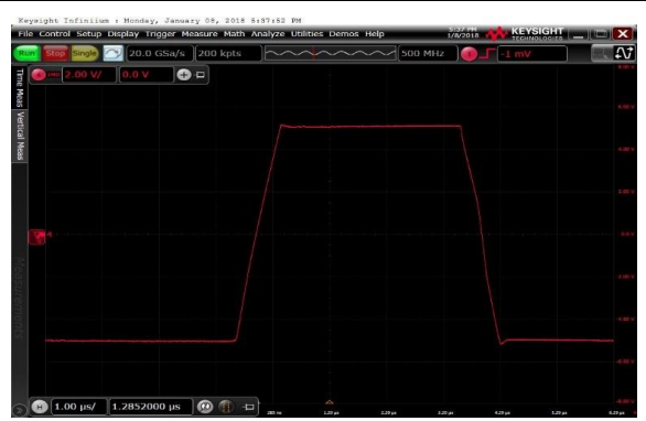
Figure 26. 10V Signal Step Response
