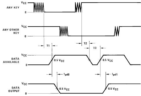
T1  $\approx$  T2  $\approx$  RC, T3  $\approx$  0.7 RC, where R  $\approx$  10k and C is external capacitor at KBM input.
