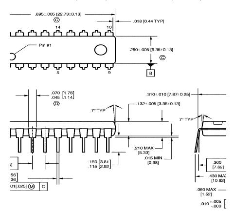
RMS TO JEDEC REGISTRATION MS-001, ONS AC, DATED 6/1993. DLLING DIMENSIONS ARE IN INCHES INCE DIMENSIONS ARE IN MILLIMETERS. OT INCLUDE MOLD FLASH OR PROTRUSIONS. LASH OR PROTRUSIONS SHALL NOT EXCEED HES OR 0.25MM. OT INCLUDE DAMBAR PROTRUSIONS
