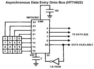
Outputs are in 3-STATE until key is pressed, then data is placed on bus. When key is released, outputs return to 3-STATE.
