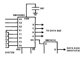
The keyboard may be synchronously scanned by omitting the capacitor at osc. and driving osc. directly if the system clock rate is lower than 10 kHz
