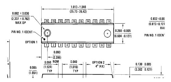
20-Lead Plastic Dual-In-Line Package (PDIP), JEDEC MS-001, 0.300 Wide Package Number N20A
